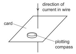
A plotting compass is placed on the card.
